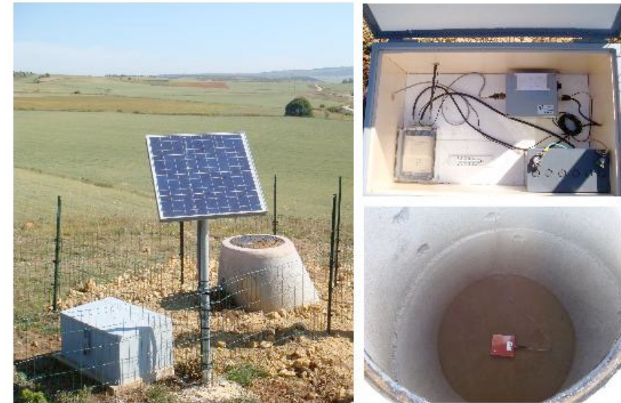
HO08 station: SARA SS-45 sensor and SARA SL-06 digitizers
